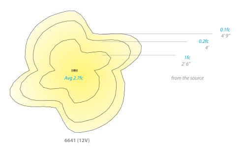
• Recommended spacing for installation :
